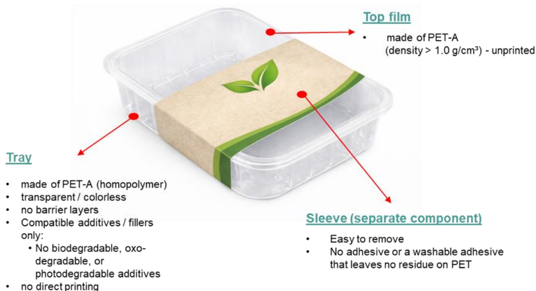
Figure 18: Option 2 – PET tray with PET top film and banderole
